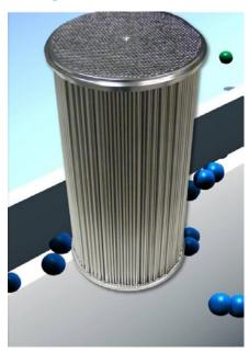
Power + Energy's hydrogen separation products use patented Palladium Alloy Micro-Channel<sup>™</sup> Technology. At elevated temperatures and positive pressures, Palladium (Pd) metal permits the diffusion hydrogen and hydrogen isotopes, but not other gases.
